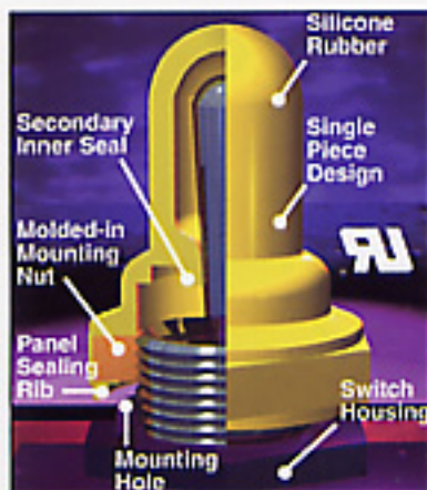
Reliable switch performance can be achieved using a separate external seal or boot.
